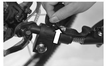
**8. Insert safety pin at the hole level.**
