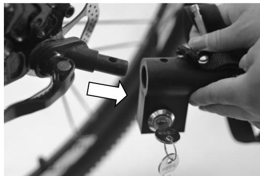
7. Insert steel connector into the hole(see picture)
