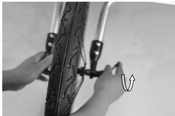
Install the front wheel in the direction shown on the front fork.
