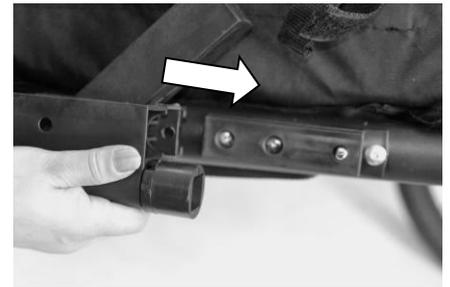
**1. Take the product out of the box. 2. Hold handle bar and pull back. 3. Install wheel holder base**
