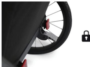
**Warning! Always apply the parking brake after parking the trailer and when getting in and out of the trailer with the children. Check that the trailer cannot roll away by pulling it slightly forwards and backwards. An unsecured trailer could cause accidents with life-threatening injuries by rolling away or could roll away when getting in or out of the trailer, causing serious injuries to the children.**
