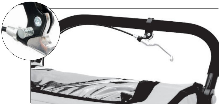
The hand brake is operated by a brake lever located on the handlebar and acts on both wheels simultaneously. To activate the parking brake, pull the brake lever towards you.
